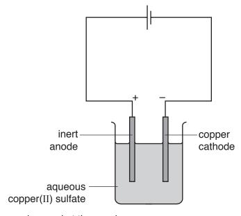
(a) Bubbles of gas are observed at the anode.
