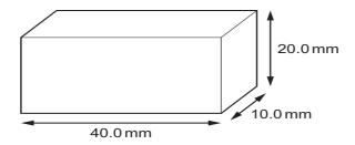
The calipers can measure with an absolute uncertainty of  $\pm 0.1$  mm.
